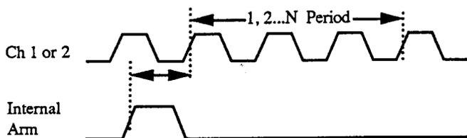
1. Period and Frequency can be measured on either channel
