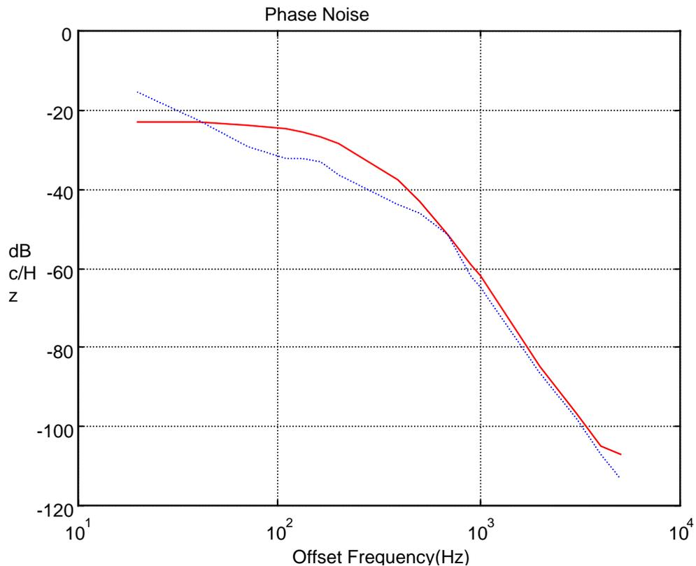
Figure 8. Phase noise measurement comparison. Solid (red) line is for HP8560E Spectrum Analyzer, and dotted (blue) line is for the DTS 2075.
