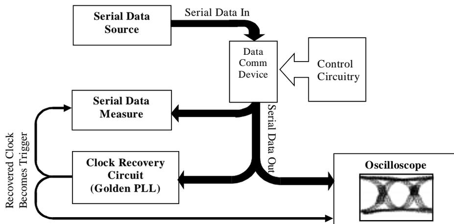
**Figure 1.1** Typical network analyzer as configured with optional Oscilloscope and Clock Recovery Circuit.
