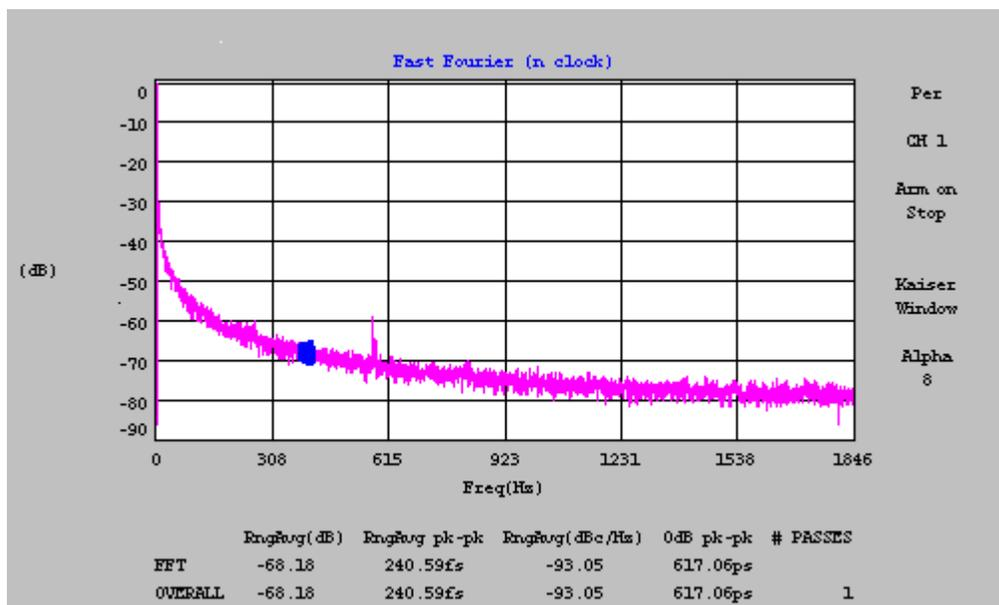
Figure 6. Time jitter spectrum as measured by the WAVECREST DTS 2075™ Time Digitizer. Phase noise at 400Hz offset frequency is shown.
