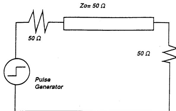
The following diagram illustrates the delay in cable measurement that results from placing a cable of mismatched impedance into the ideal model.
