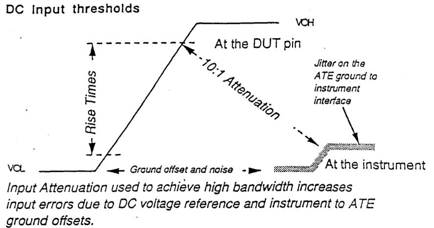
A high ATE system jitter noise floor masks real DUT performance. Most ATE systems specify 20ps to 50ps rms jitters. For Telecom work rms jitter must be multiplied by 6 to 8 to get 6 to 8 sigma results. That means the ATE system at 50ps rms jitter is really 300ps to 400ps of peak-to-peak jitter! Consequently, for such measurements an instrument with 5ps rms jitter or less is necessary.
