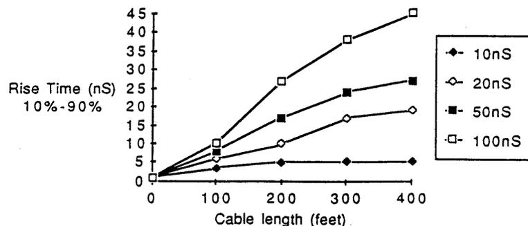
Amplitude is attenuated as cable length increases. The following diagram illustrates peak amplitude attenuation versus cable length.
