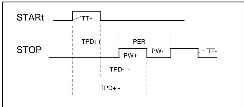
Waveforms Diagram of the DTS2010 nine acquire function modes.
