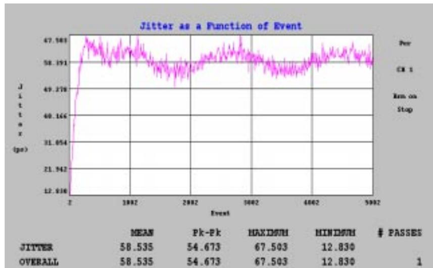
Figure 3 - Accumulated Jitter
