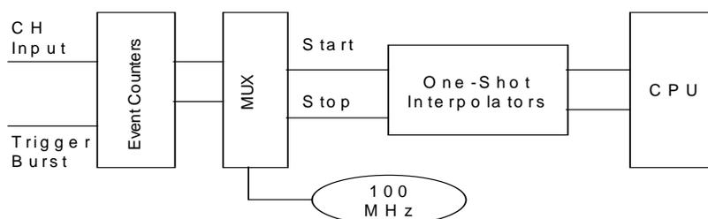
Figure 4. A schematic for DTS system architecture
