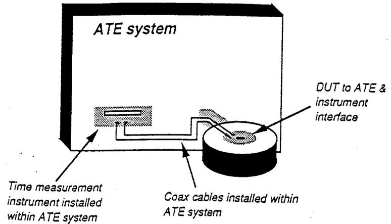
LSI and VLSI ATE systems normally have room within the confines of the system cabinets for external instruments. Most of these systems also have high quality  $50\Omega$  coax cables running between the instruments and test-head load-board interface hardware. Some systems have special coax pogo-pins to make contact to the DUT board. This level of integration is recommended for an accurate low jitter production and engineering environment.
