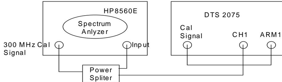
Figure 7. Experimental set up for RF Spectrum Analyzer and DTS 2075 to measure phase noise for a common input signal.
