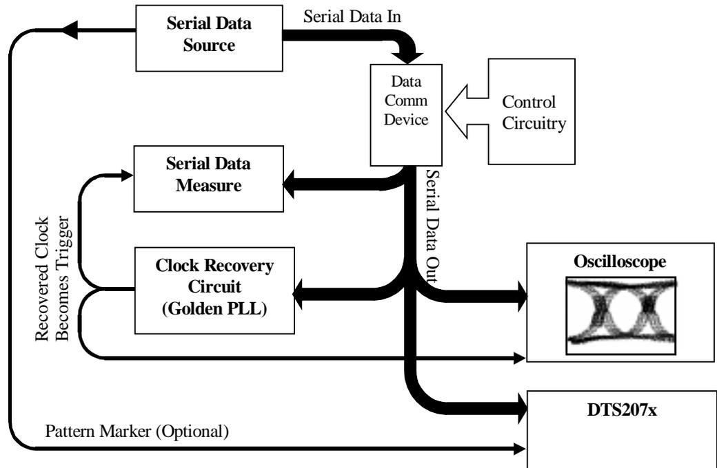
**Figure 1.3** Typical Network Analyzer and DTS 207x setup.
