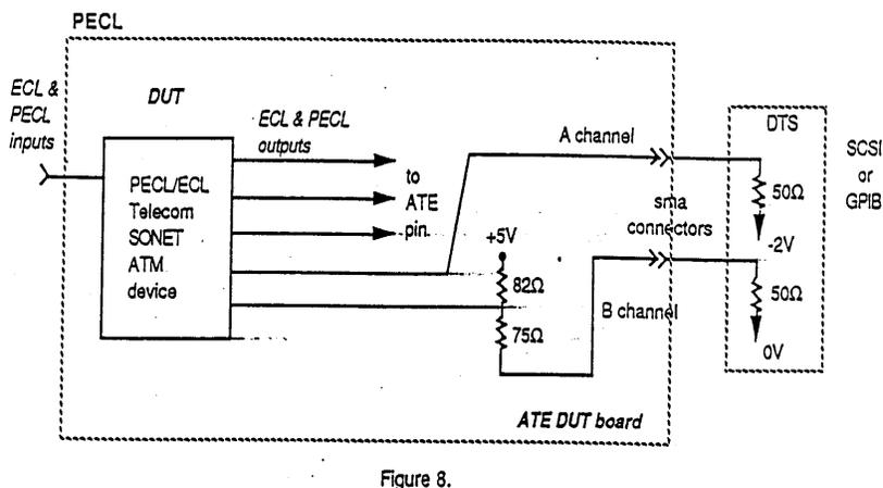
Figure 8 shows a PECL-to-ground reference level shifter. Chip resistors and capacitors minimize parasitic reactance. High quality 50Ω coax cable is required to transfer signals to the time measurement instrument.
