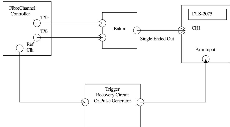
**Figure 1 - Instrument Setup**
