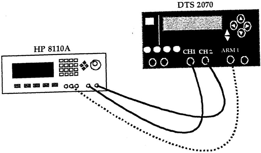
Pulse generator setup for delay measurements
