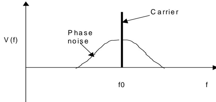
Figure 2. Spectrum of a sine wave with phase noise.
