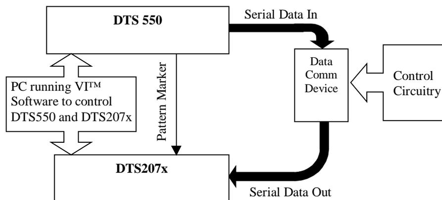
**Figure 1.2** *WAVECREST* Data Communications characterization setup.
