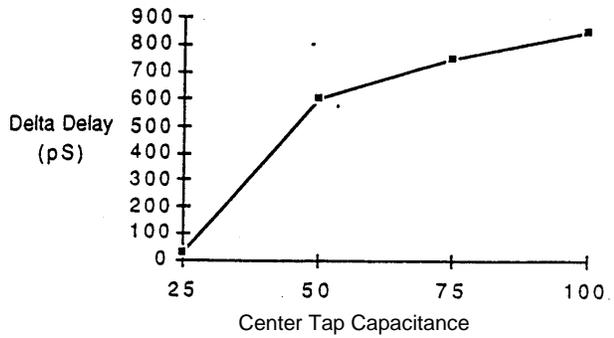
The following diagram illustrates an actual series of measurements, showing the delay in cable measurement that results from placing a cable of mismatched impedance in a test setup.
