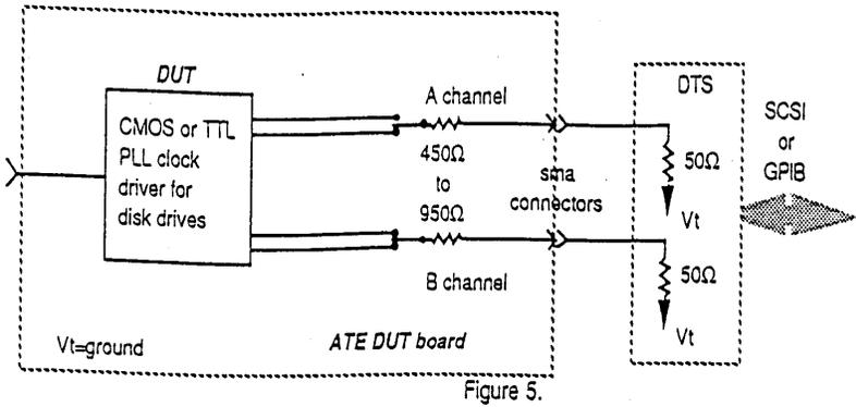
Figure 5 shows an interface implementation where the external instrument makes the voltage and timing measurements. No connection is made to the ATE system for the PLL clock skew pins. The ATE system provides OUT power and pattern stimulus.
