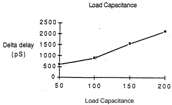
The following diagram illustrates the change in delay readings when a capacitive element is introduced into the middle of the ideally-matched cable.
