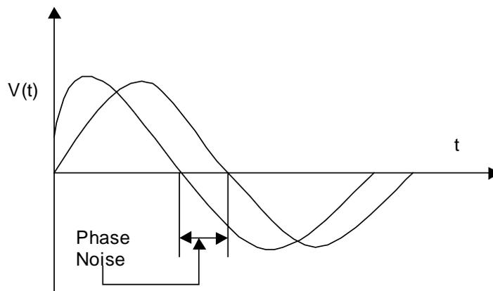
Figure 1. Illustration of phase noise.
