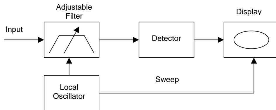
Figure 3. Sweeping Spectrum Analyzer.
