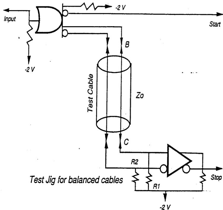
This example is another variation on the previously illustrated substitution techniques (see Bench Setup). The input of the cable test set, A, fed by an ECL level signal, is terminated to -2 volts, and provides a 50 ohm impedance match. This input can be fed with a signal generator. The 100112 buffer splits the signal, one for the Start input of the DTS, and the other for the Stop input.
