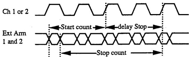
1. The count can be used to delay the Arm event or the Channel on either channel for both Start and Stop.
