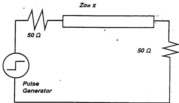
The following diagram illustrates the change in delay readings when the terminating impedance is mismatched.
