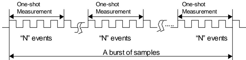
Figure 5. A schematic of the Time Digitizer function.
